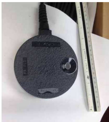
This embedded so-called hockey puck relays roadway weather data.
